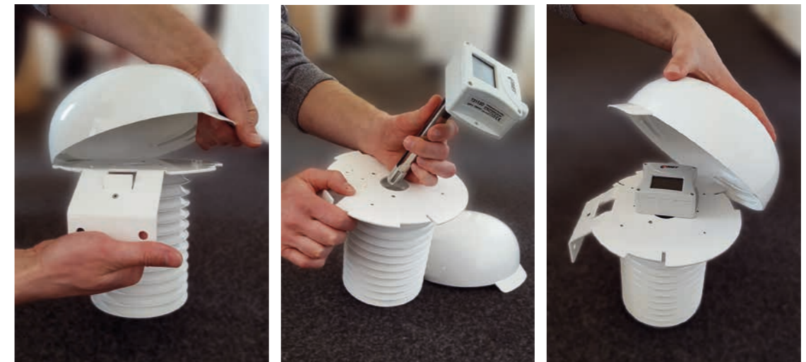
Mounting of sensor inside of COMETEO.
